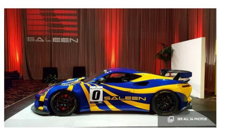
The GT4 concept features updates to its front splitter and fenders, plus a new rear diffuser to improve aerodynamics. Per GT4 specifications, a large rear wing adds downforce. The concept car also offers front and rear ABS and other GT4-specific equipment.
